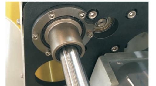
4 Spline gearing device
